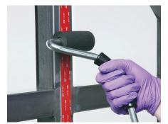
STEP 3: Apply pressure with a J-roller to at least 15 psi (100 kPa). This will help develop highstrength adhesion and bonding. Bond strength will increase after application.
