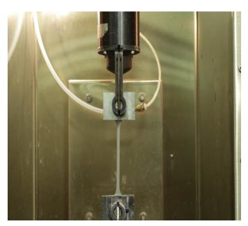
Tensile and elongation tests: Used to compare 3M VHB Tape's elongation versus adhesives. Unlike traditional joining methods, 3M VHB Tape can isolate stresses by allowing them to move independently, while still maintaining a strong hold.
