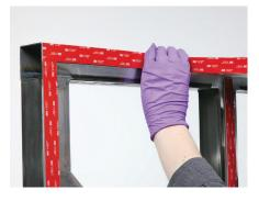
**STEP 2:** When surfaces are dry, apply 3M VHB Tape to the surface.
